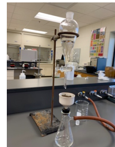
Figure 4. The apparatus used to extract nitrate from the soil samples is shown.
