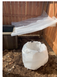
Figure 2. The passive warming device is shown at the bottom of the picture. Shown at the top is the plastic sheeting draped over an area to decrease precipitation.
