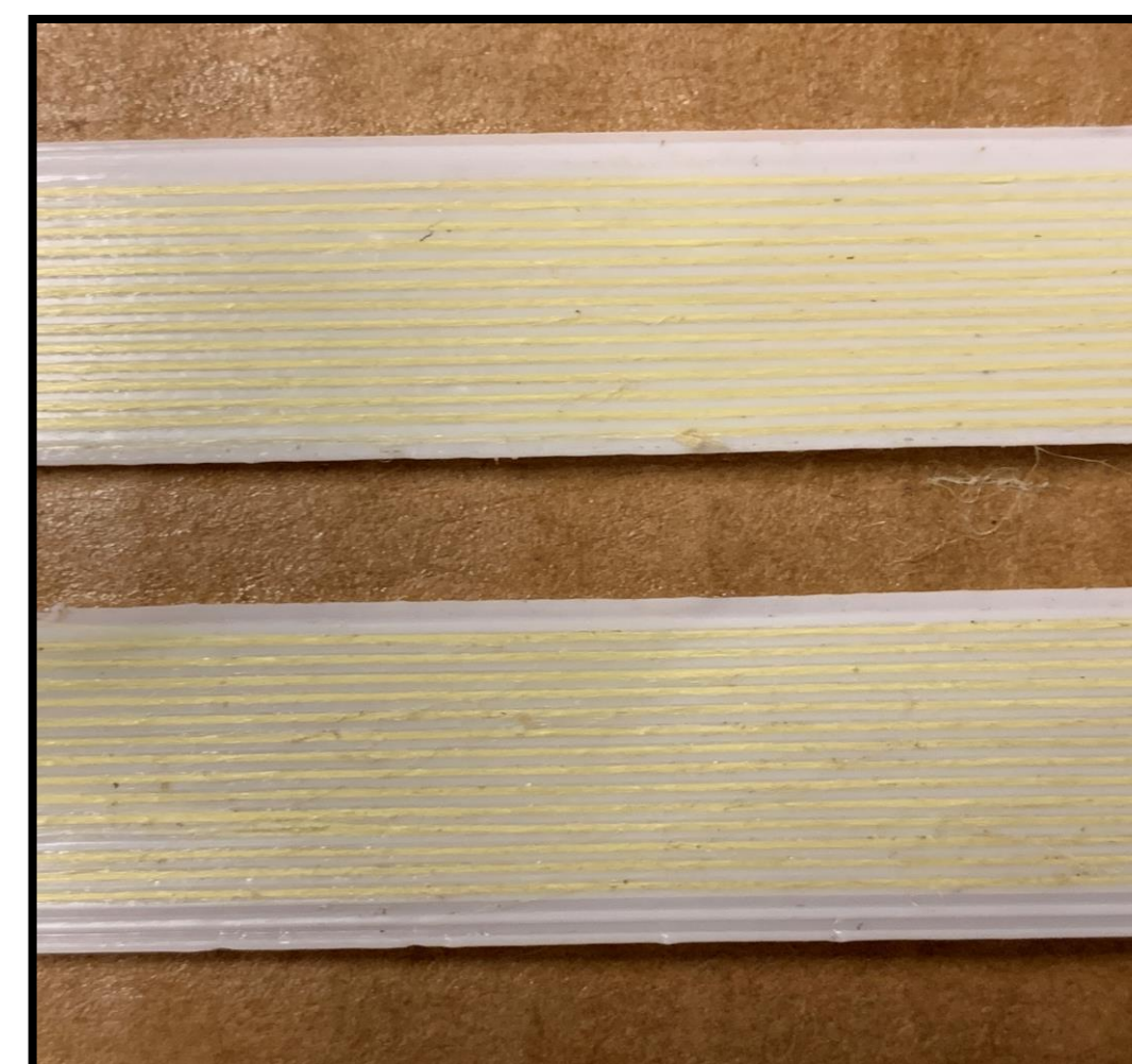
Rows of printed PLA plastic showing successful deposition of Kevlar strands
