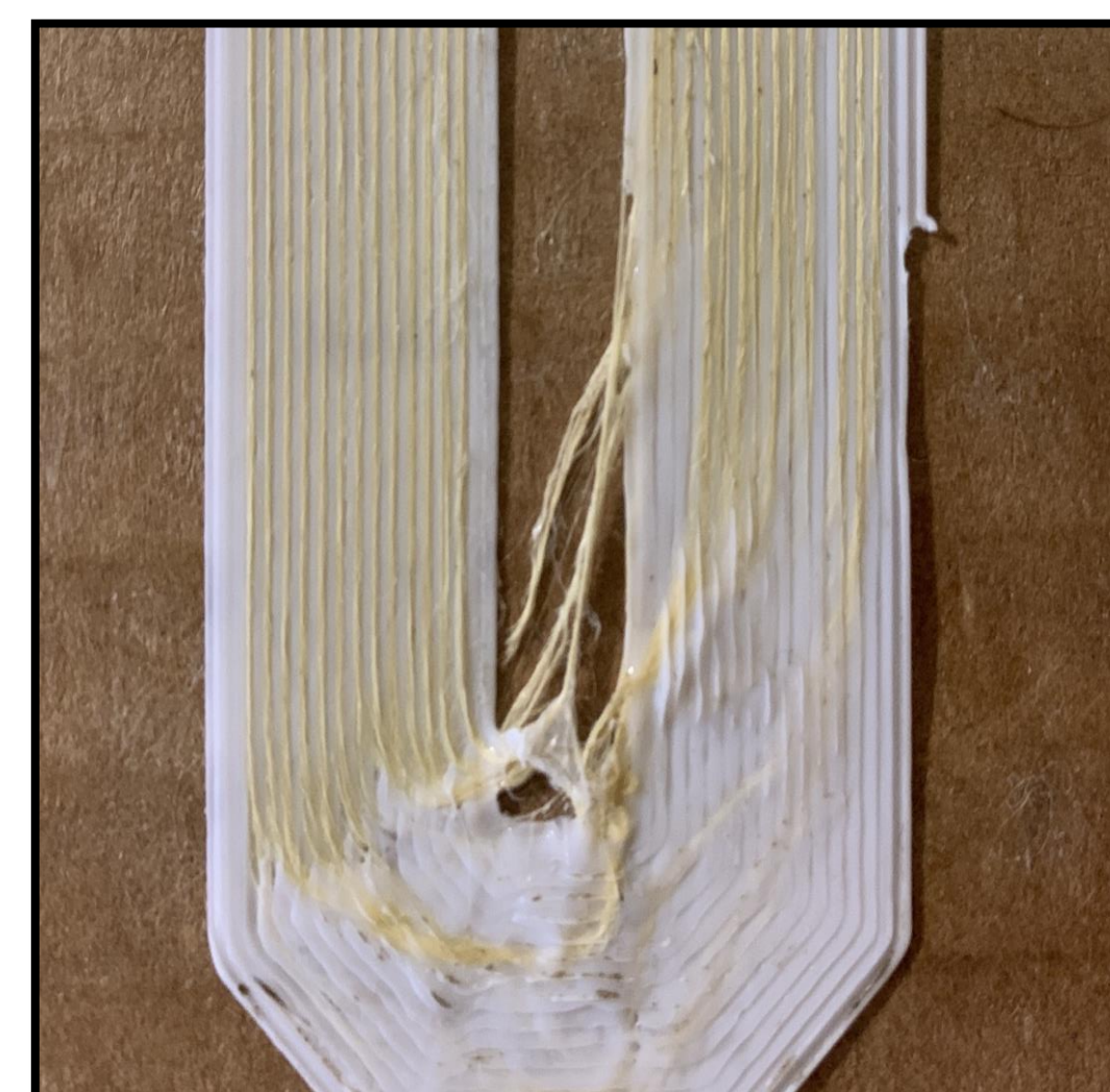
Fiber that was pulled out of sync on a sharp corner. This was the primary problem encountered in this research.
